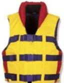
The Type III foam vest has the same minimum buoyancy as a Type II. It comes in many styles, colors, and sizes and is generally the most comfortable type for continuous wear. Float coats, fishing vests, and vests designed with features suitable for various sports activities are examples of this type. This type of inflatable turns as well as a Type II foam vest.
