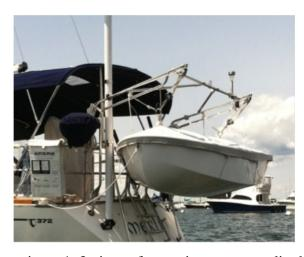
using a 1x3 piece of strapping, onto my dinghy and then put the set in my storage bin. In the spring I reverse the process once Merlin gets back on the mooring. Another option is to have your davit arms swing together once the top span bars are removed. Unfortunately with my rear radar post, this was not possible for me.
