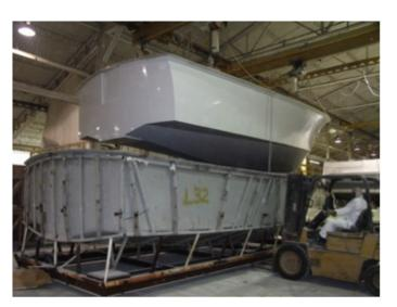
Legacy 32 fully pulled from the hull mold
